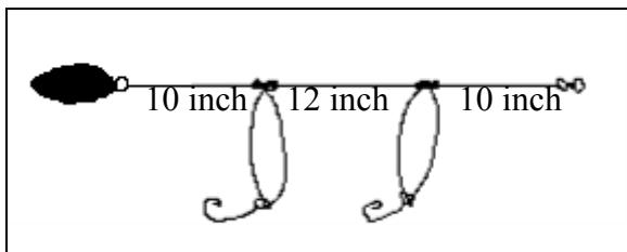
The running rig is a good rig for calm conditions. The sinker can sit on top of the sinker or the swivel and can be 1/4oz up to 6oz depending on conditions
